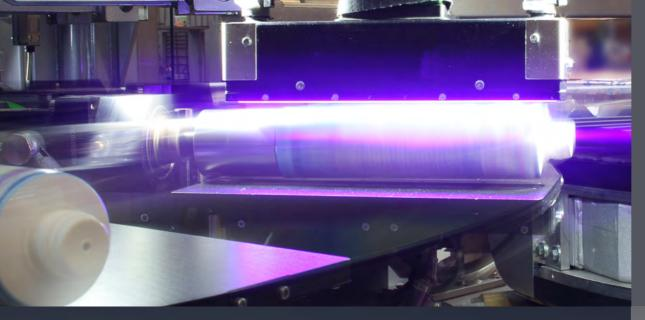
Precise surface treatment, pin and final UV LED curing
